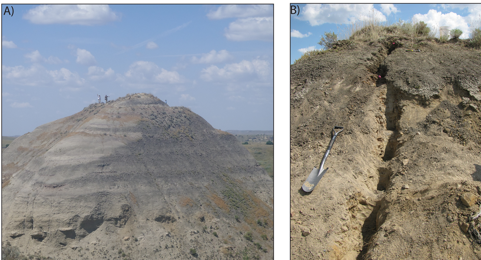
Figure 1. A) Butte east of Marmarth, ND. Sediment samples were collected from the upper 1/3 of the butte. B) Partial image of the stratigraphic section dug into the south side of the butte. Digging a section in this manner ensures that horizontal strata, rather than slumped sediment, is sampled. Pink markers in the section indicate changes in strata.
